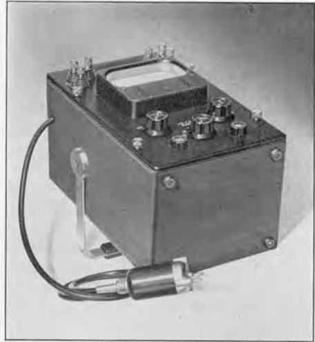
Figure 6. As shown here, the voltmeter can be used with the panel inclined, support being provided by the handle, which locks into position.
