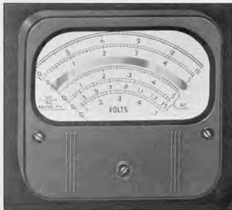
Figure 2. Close-up of the meter scales. The legend at the left is carried to the top two scales by a line that, in this view, is hidden by the meter case.
